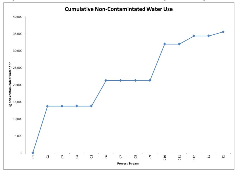
Graph of Cumulative Non-Contaminated Water Use / Emission through Manufacturing Process
